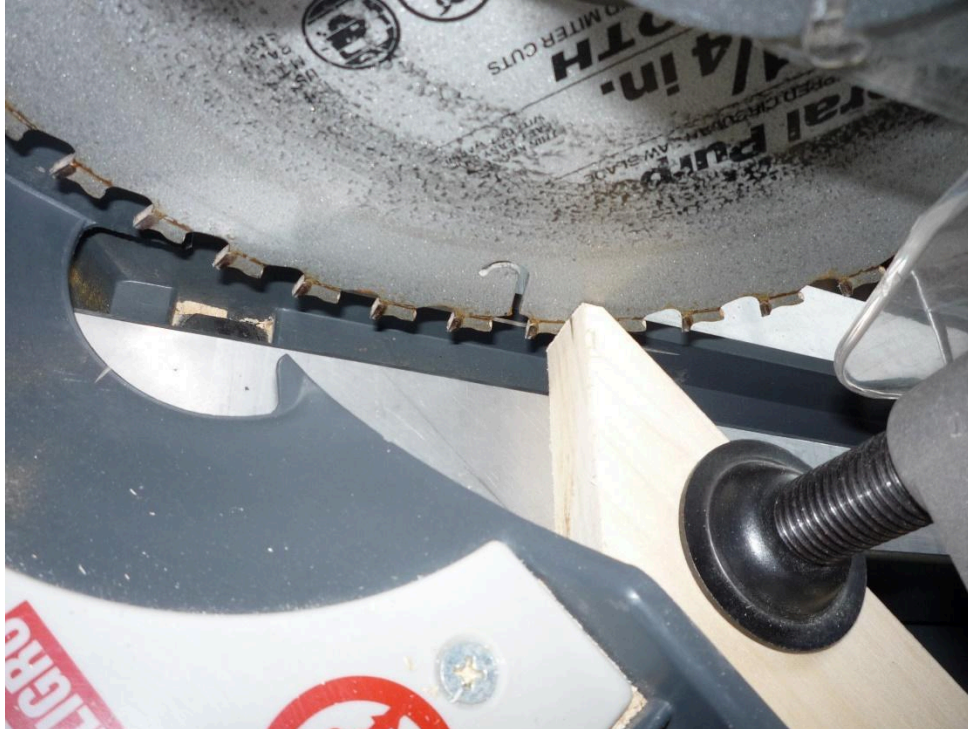
“back cut” the 45 degree angle, and sand the leg ends to minimize splitting
